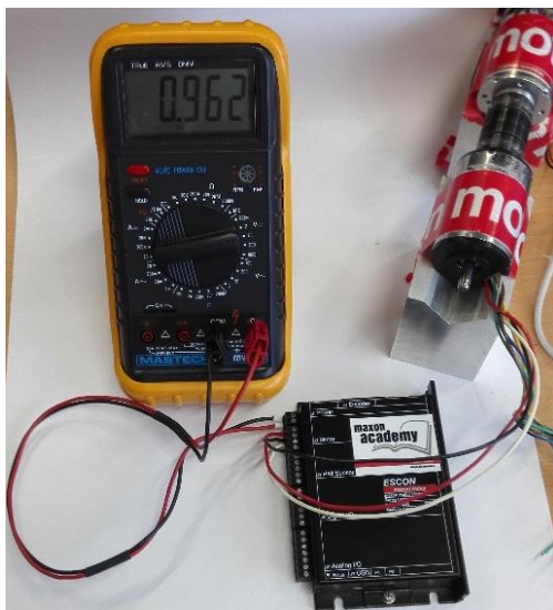
Figure 8 Using an ESCON as a rectifier. Connect the 3 motor phases. The generated voltage can be measured at the ESCON power supply input.
