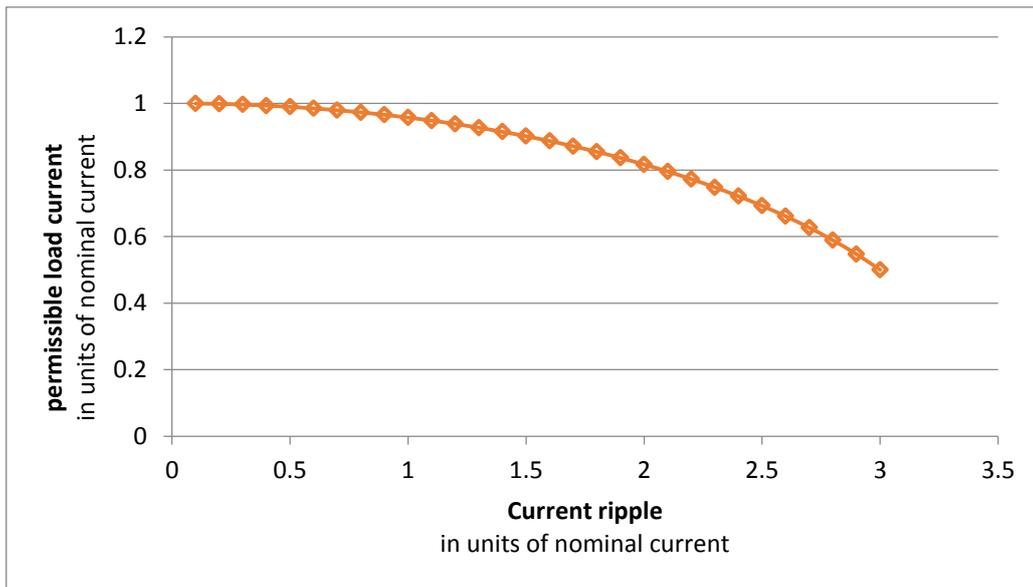
From the chart one can see that at a peak-to-peak current ripple of 1.5 times the nominal current the motor should only be loaded by about 90%. This implies that quite large current ripples can be tolerated from a thermal point of view, without losing too much motor performance. And never forget, that's the worst case scenario with 50% PWM duty cycle (in case of a 3-level PWM switching scheme), i.e. running the motor with half the supplied voltage.
