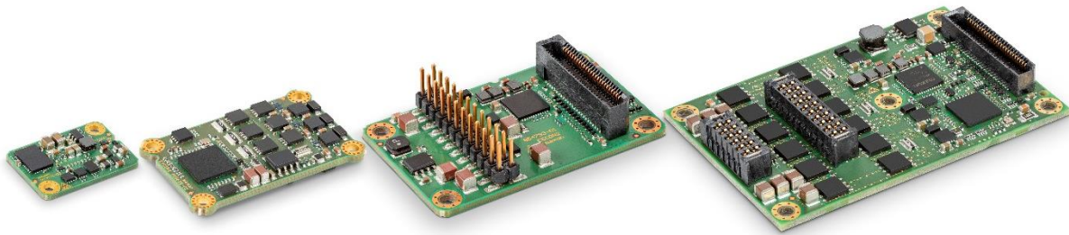
«ESCON2 Nano 24/2» (P/N 809635) 23 × 16 × 4.5 mm, 2.5 g «ESCON2 Micro 60/5» (P/N 809631), 36.8 × 23.8 × 6.5 mm, 6 g «ESCON2 Module 60/12» (P/N 854796), 49.5 × 31 × 12.4 mm, 12 g «ESCON2 Module 60/30» (P/N 783722), 67 × 43 × 7.8 mm, 19 g
