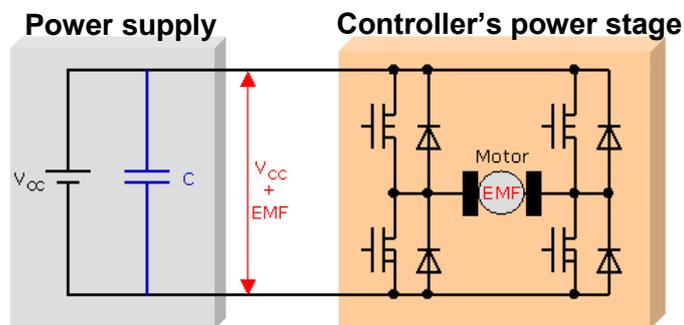
The maximum occurring voltage depends to a high degree on the supply voltage  $V_{cc}$  and the speed  $n(0)$  at the beginning of the braking. Further influencing factors are the total mass inertia  $J_{tot}$  and the achieved deceleration rate  $a_{brake}$ .
