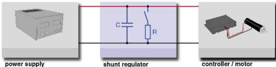
There can be one shunt regulator in use for multiple drives depending on the amount of reversed energy. The shunt regulator has to be placed in the supply voltage line in between the power supply and the controller.
