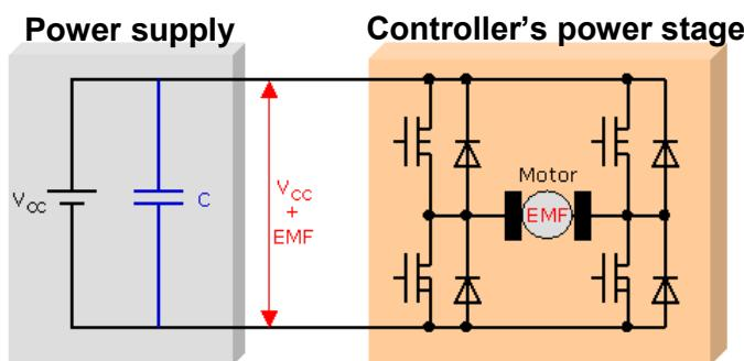
The maximum occurring voltage depends to a high degree on the supply voltage  $V_{cc}$  and the speed  $n(0)$  at the beginning of the braking. Further influencing factors are the total mass inertia  $J_{tot}$  and the achieved deceleration rate  $a_{brake}$ .
